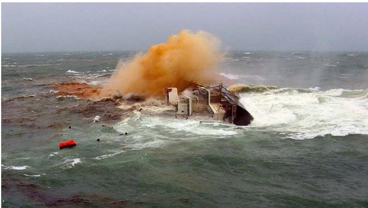
Bulk Carrier 'Trans Summer' capsizes due nickel ore liquefaction during Typhoon Utor, Aug 2013 Photo: HKG Flying Service
