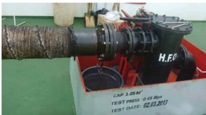
The initial overflow will be contained within permanent steel save-alls which (as depicted in the adjacent photo). must be fitted around bunker air vents and manifolds. However, the capacity of these save-alls is relatively small and they can be filled within seconds to then overflow to the maindeck. If maindeck drain scuppers have not been securely plugged, the
