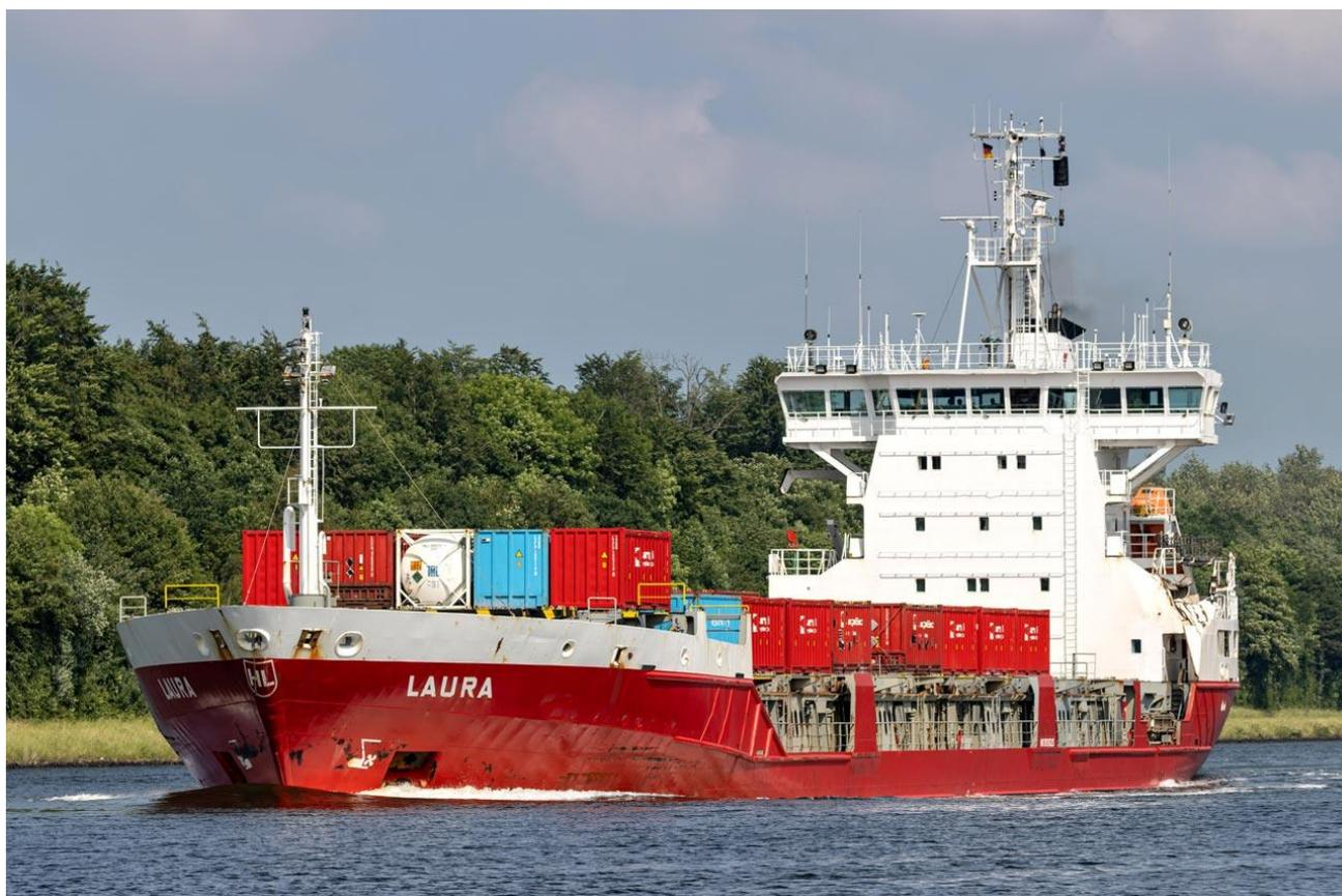
MV Laura – a non-cellular ‘General Cargo’ vessel (GT 5329) with containers loaded on to the hatch covers.
