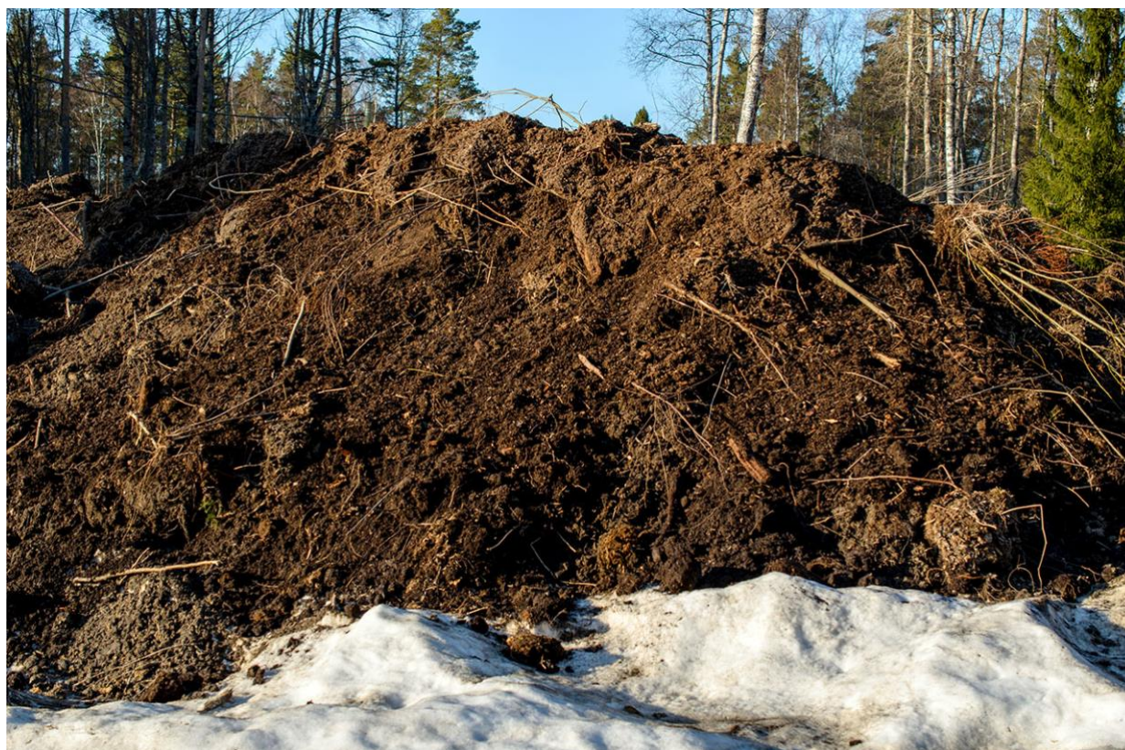
Excavated soil: not listed in the IMSBC Code, but potentially a Group A (may liquefy) bulk cargo.
